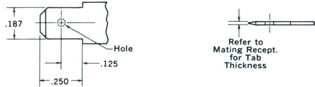
MATING 187 SERIES TAB DIMENSIONS
